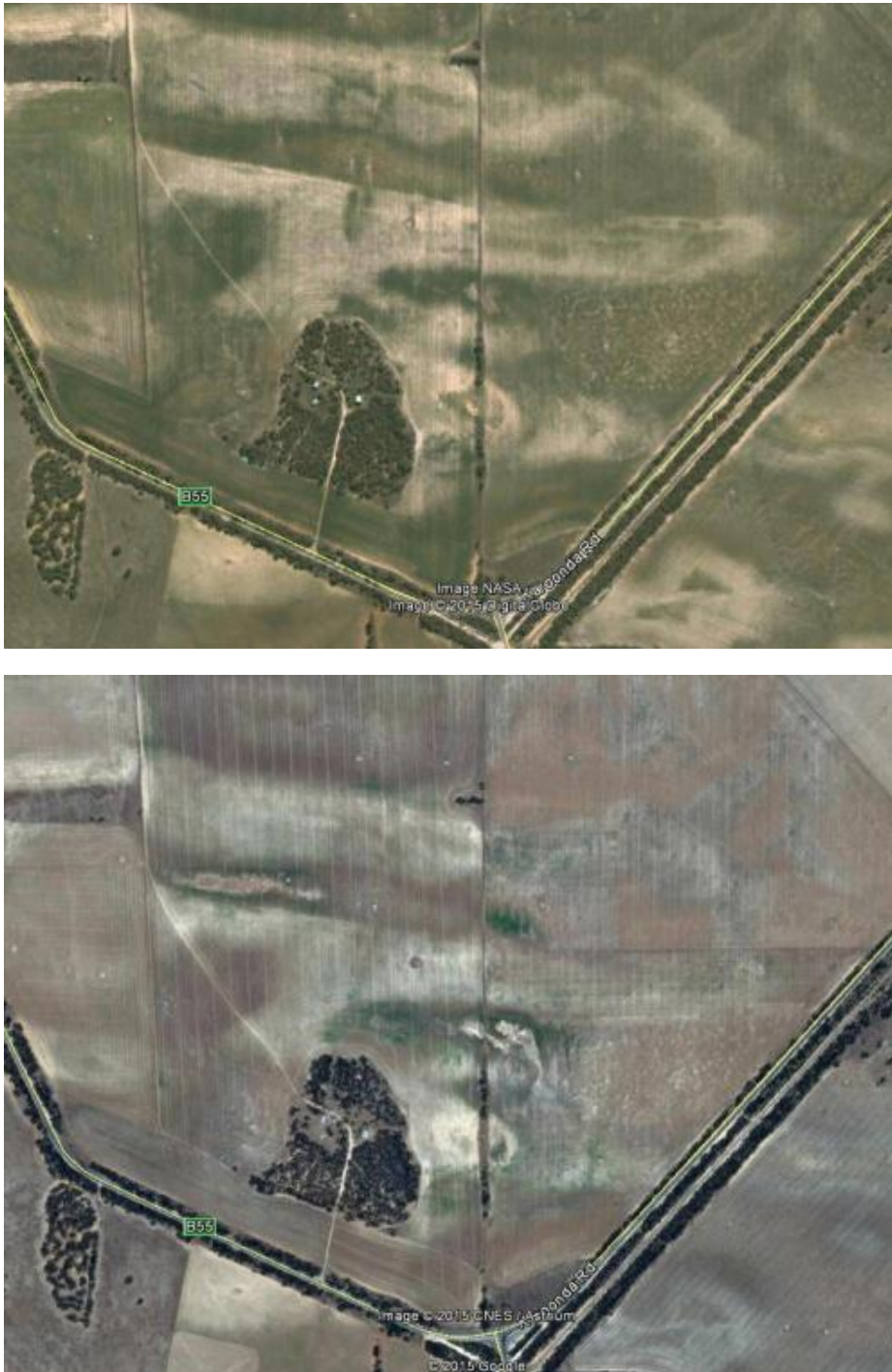
Figure 22: Satellite imagery showing seep development between 2006 and 2013 (GoogleEarth™, 2015)
