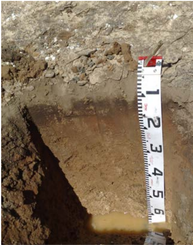
Figure 24: Shallow watertable exposed underneath bare area, Wynarka October 2011
